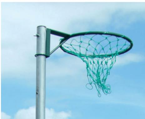
Uprights manufactured from 50mm diameter x 1.6mm thick plated steel with punched hole which allow hoops to be adjusted to 2.5mm, 2.6mm, 2.7mm and 3.05m heights. Triangular base which doesn't protrude into the playing court, complete with double Nylon wheels and rubber pads for floor protection. Complete with 10mm solid steel hoops and rings.
